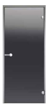
The aluminium frame door is an excellent solution for a steam room or a sauna door. It is designed for conditions where the materials need very good humidity resistance. There are no wooden parts in the door. The aluminium frames  $(40 \times 60 \text{ mm})$  are light grey in colour. The glass is tempered 8 mm safety glass. Seals keep the heat and steam in. Aluminium frame door is maintenance-free decade after decade.
